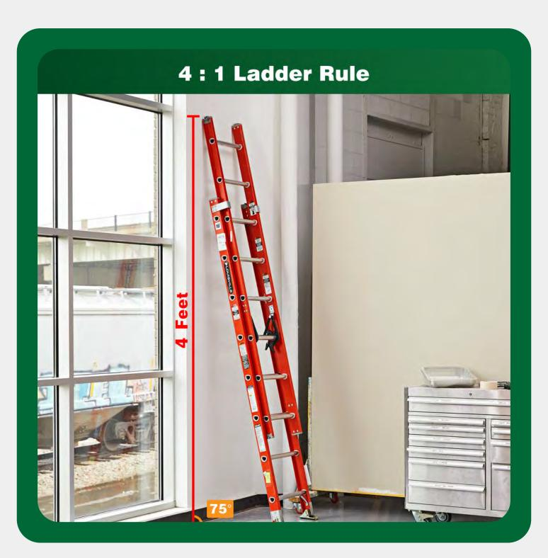
For every four (4) feet of height you climb, move the base one (1) foot away from the wall that the ladder is resting against.
